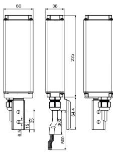
Preassembled oilflex-sheathed cable (classic 100): 8 (for 1 relay) or 9 (for 2 relays) x 1 mm<sup>2</sup> with ferrule on bare end of core on connection side
