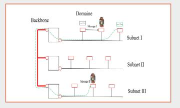
If we now bring together both ideas of **full duplex data transmission** and a **suitable protocol** that allows structuring, the result is a new technical solution that goes far beyond what is available today in the field of wireless communication. Considering the LON specification and its limitations, it is theoretically possible to build networks in a domain with 255 subnets and 127 controllers per subnet.
